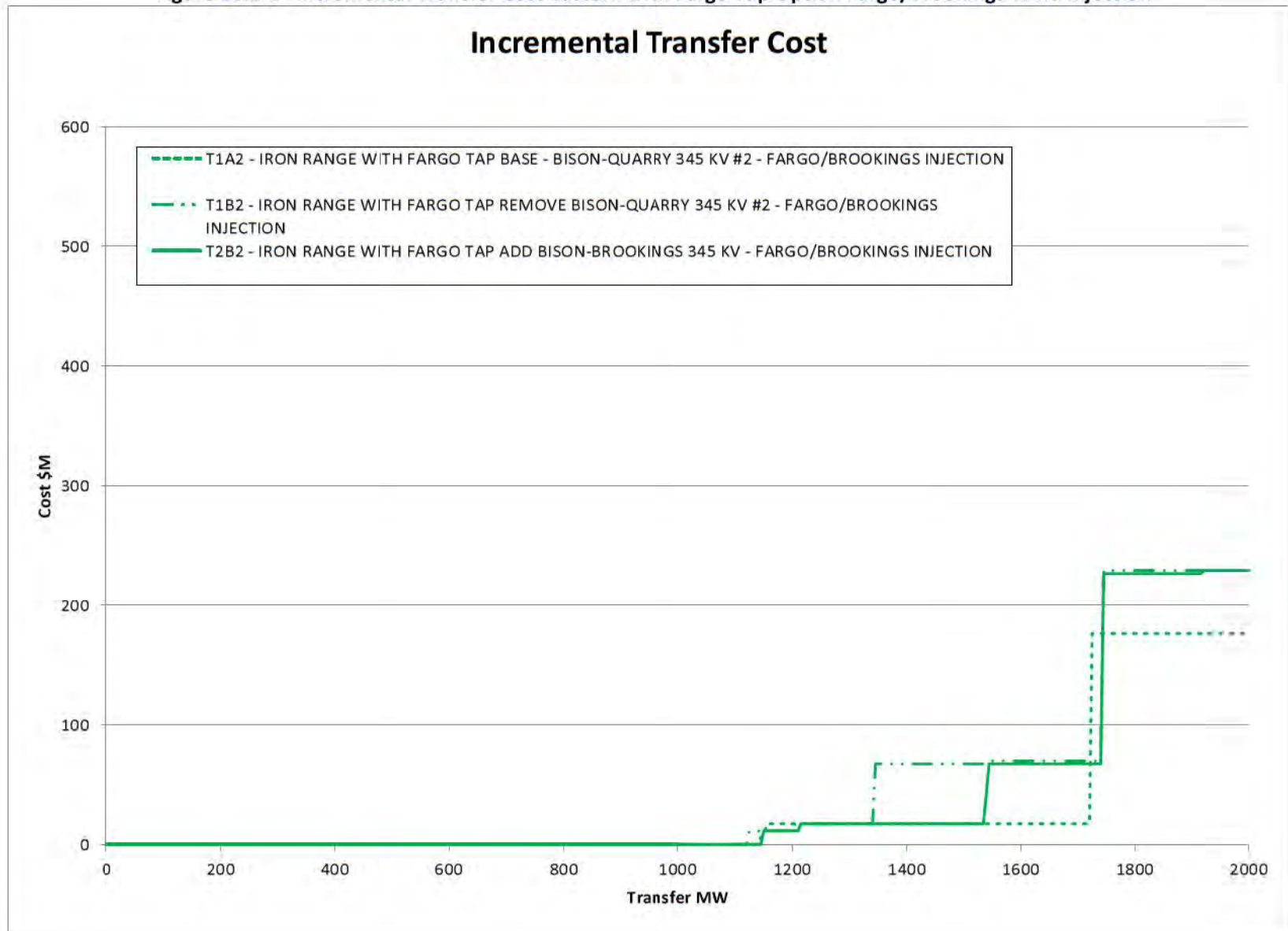
Figure E3.2-1 Incremental Transfer Cost Eastern with Fargo Tap Option Fargo/Brookings Wind Injection
