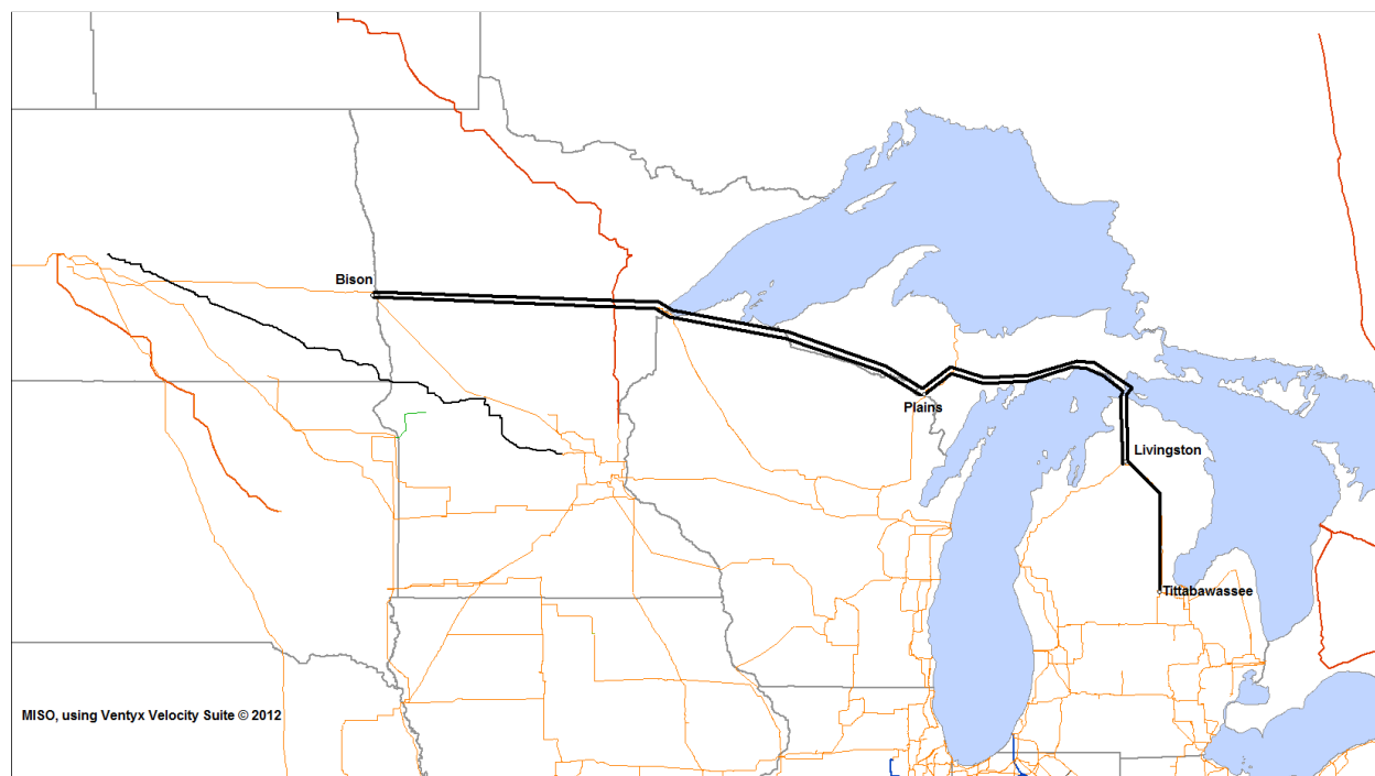
Figure 6-38: Bison – Plains – Livingston/Tittabawasse 500 kV HVDC
