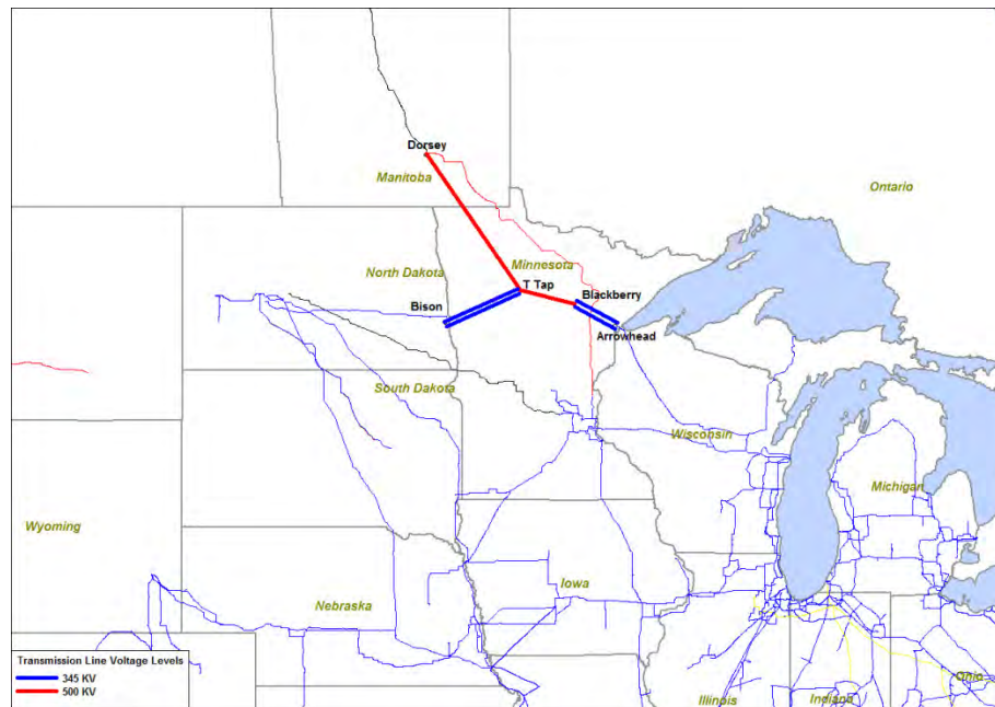
Figure 1-5: Manitoba – Fargo and Duluth “T” 500 kV Tie-Line
